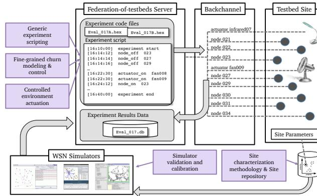
Fig. 1. Overview of the elements that are planned to be introduced to support realism and reproducibility (left), and where they influence the process of evaluating particular WSN code: The nodes' firmware is submitted to the server along with an *experiment script* that allows *fine-grained churn control* as well as *controlled environment actuation*. A set of *testbed site characterization* parameters are fed back together with the raw output data after the experiment.
