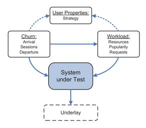
**Fig. 20.1:** P2P system under test. The *system* is controlled by the *workload* and *churn* components. Different users are modeled by *user properties*. Finally, the *underlay* decides about the transmission delays.
