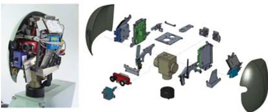
Figure 2. Explosion view of the head-components
