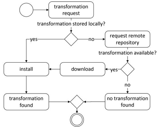
Fig. 3. Processing an event transformation request: If there is no transformation from the advertised event type(s) to the required event type stored locally, the request is forwarded to a remote transformation repository allowing the system to adapt to new requirements.
