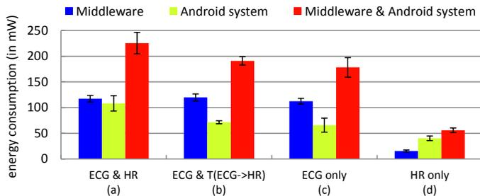
Fig. 10. Energy consumption for different sensor constellations. Having a transformation converting ECG streams to heart rate data (b) saves more than 15 % energy compared to having both sensors connected (a). Compared to an ECG sensor (c), a heart rate sensor (d) consumes perceptible less energy.
