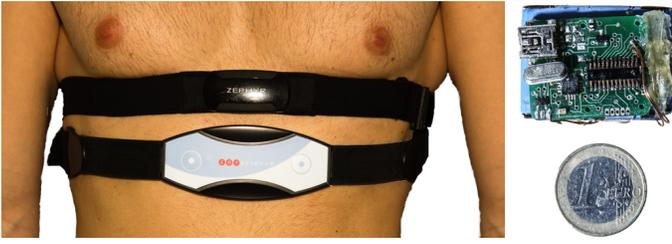
Fig. 6. A Zephyr HxM Bluetooth heart rate sensor and a Corscience CorBELT Bluetooth 1-lead ECG sensor were used for testing the  $T_{ECG \rightarrow HR}$  transformation and energy consumption. The HedgeHog sensor on the right provides acceleration data for the activity recognition needed in  $T_{HRA\text{alarm}}$ .
