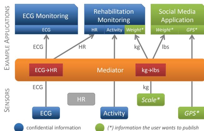
Fig. 1. Illustration of a mediator for patient monitoring that delivers only the desired and permitted readings and transforms readings from one data representation to another which obviates the need for some sensors (e.g., HR).
