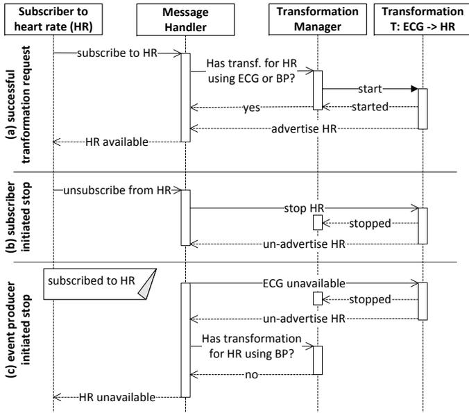
Fig. 4. Sequence diagram illustrating the communication among software components for starting and stopping an event transformation: (a) installing an event transformation for transforming events of type ECG to type HR, (b) the event transformation is stopped because the last subscriber to HR unsubscribed, (c) the event transformation is stopped because the event producer for events of type ECG is no longer available.
