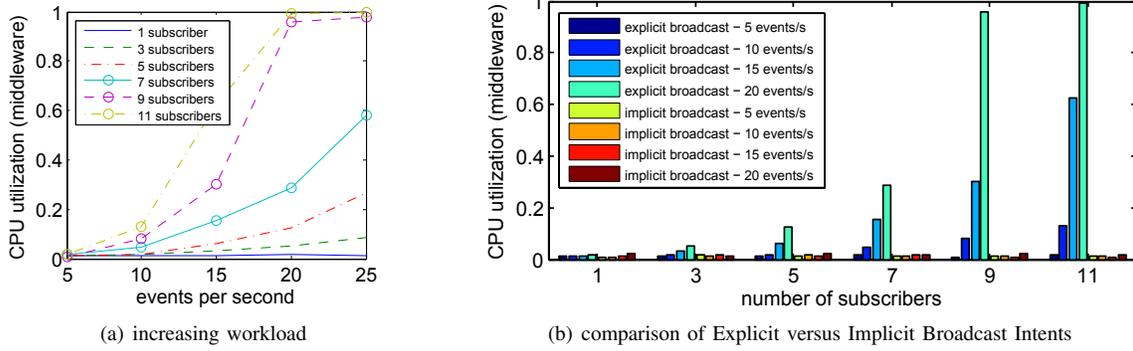
Fig. 7. CPU utilization of the middleware for (a) an increasing number of events/s, and (b) an increasing number of event subscribers.
