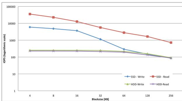
Figure 3: Random throughput HDD, SSD
