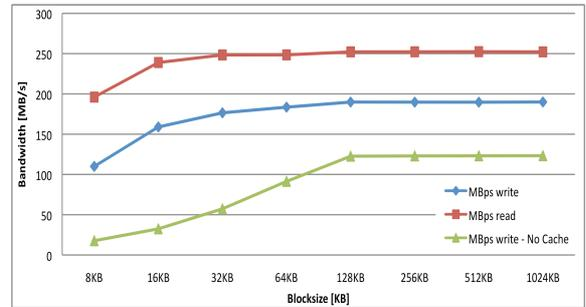
Figure 2: Sequential throughput (MB/s)
