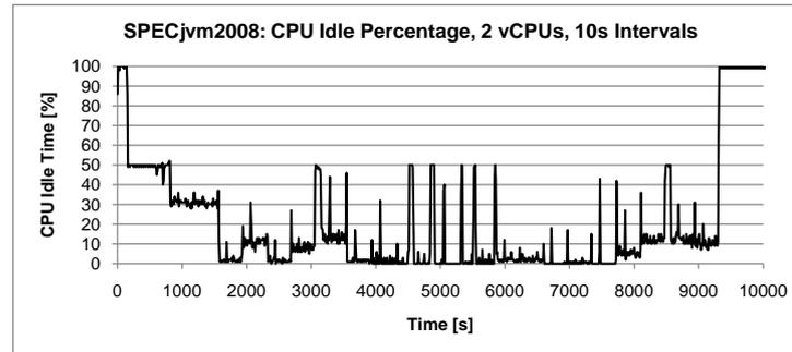
Figure 2. CPU Idle Time during SPECjvm2008 Run
