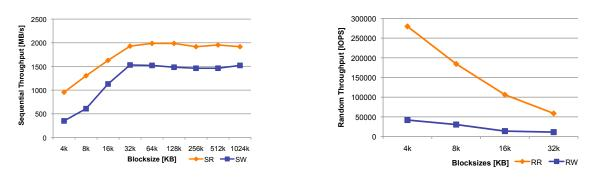
Fig. 3. Measured sequential throughput
