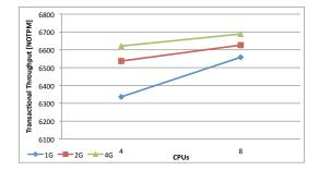
Fig. 10. Increase in transactional throughput (NoTPM) for different number of CPUs (buffer size - constant, page size 4KB)
