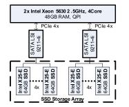
Fig. 1. Experimental testbed architecture
