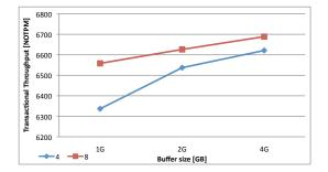
Fig. 9. Increase in transactional throughput (NoTPM) for different buffer sizes (number of CPUs - constant, page size 4KB)
