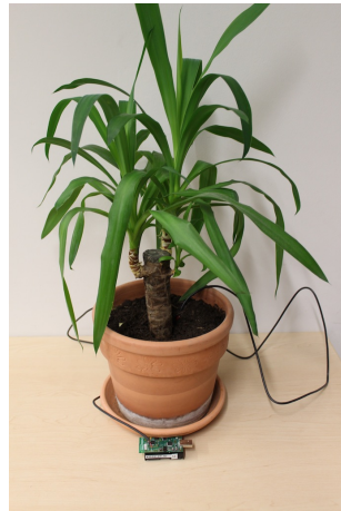
Figure 3.12: Plant monitoring using a VH400 soil moisture sensor mounted on a TelosB node.
