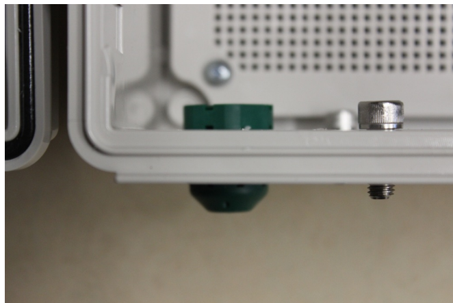
Figure 3.6: The vent plug mounted in the enclosure.
