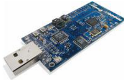
Figure 3.10: TelosB ultra-low power wireless module.
