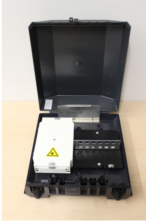
Figure 3.8: A fiber-optic passive distributor manufactured by the R&M company.
