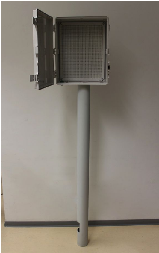
Figure 3.5: First prototype of the stations: The enclosure mounted on a pipe.
