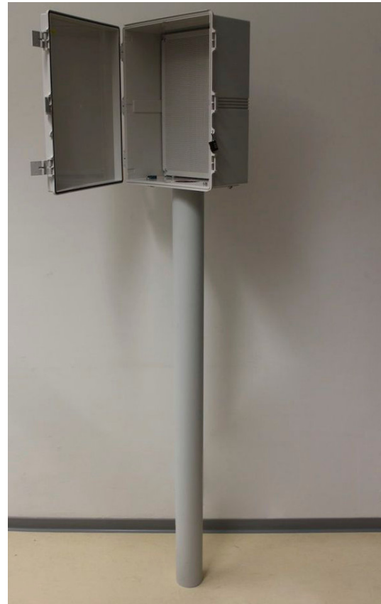
Figure 3.5: First prototype of the stations: The enclosure mounted on a pipe.
