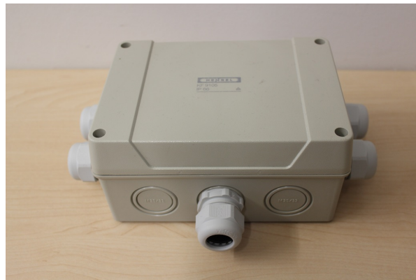
Figure 3.9: The Hensel cable junction box used as a power splitter in the two main stations .
